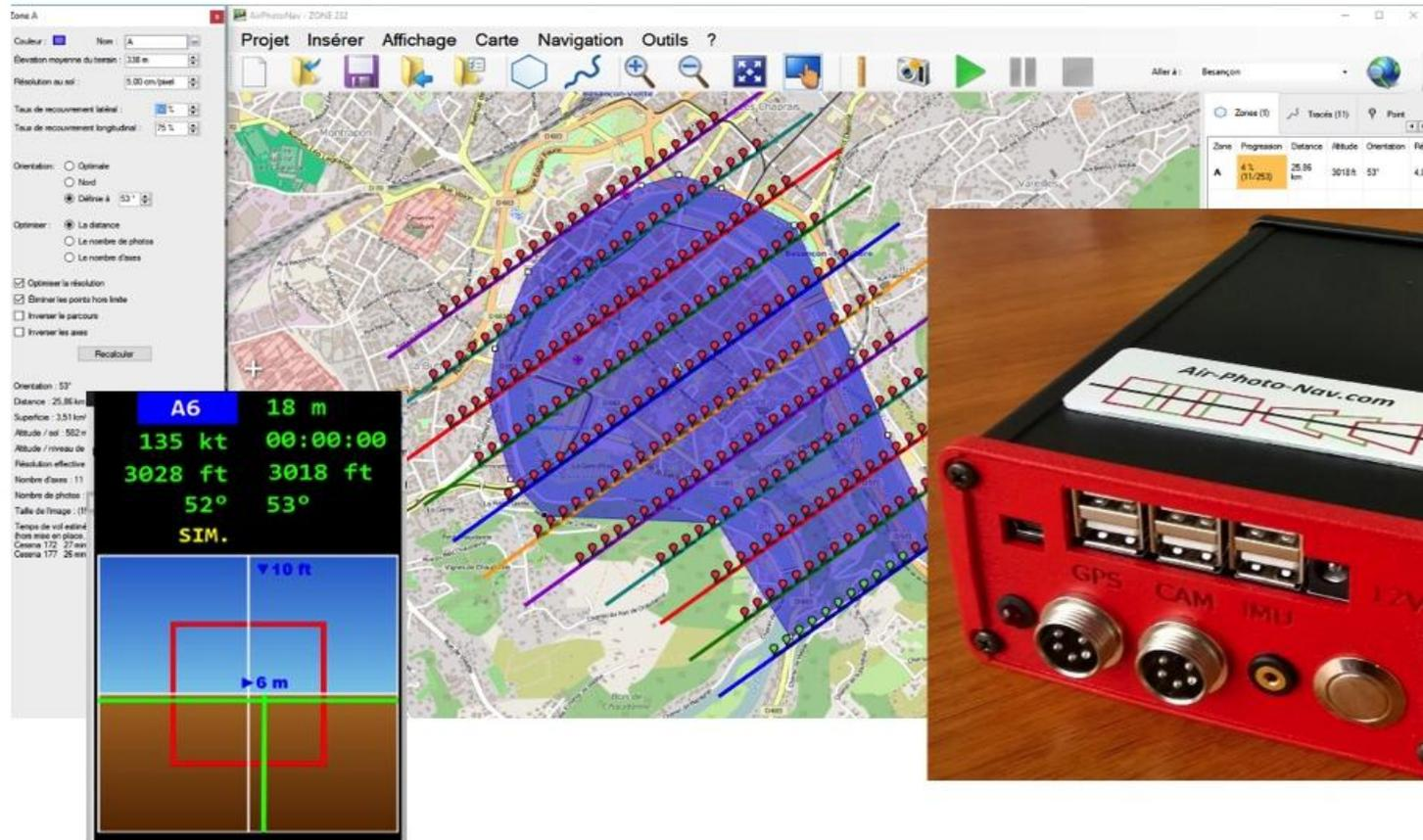
The screenshot displays the Air-Photo-Nav software interface. The main window shows a map with a flight plan overlaid, consisting of several parallel flight lines with waypoints. The left sidebar contains various settings for the flight plan, including orientation, optimization, and resolution. A technical data panel in the bottom-left corner provides the following information:
